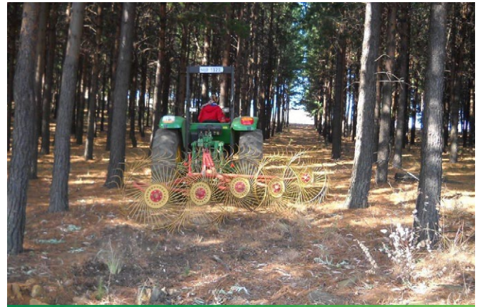
Figure 18: A belt created by raking the area clean of loose material
