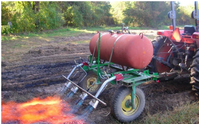
Figure 26: Tractor-mounted flamethrowers used to incinerate green plant material
